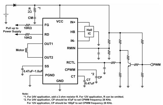
Figure 1. TSSOP -16 24V and 12V Typical Application Circuit
