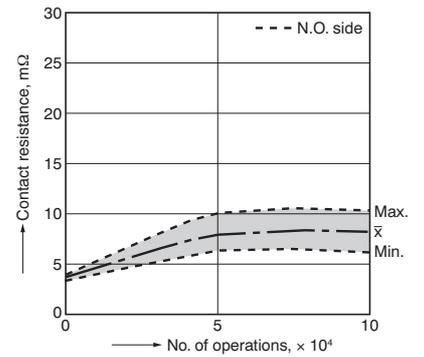
5.-(2) Electrical life test (Lamp load)
