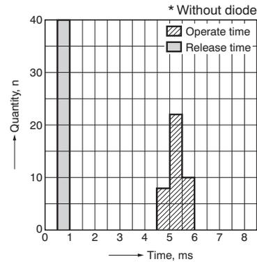
5.-(1) Electrical life test (Motor lock)
