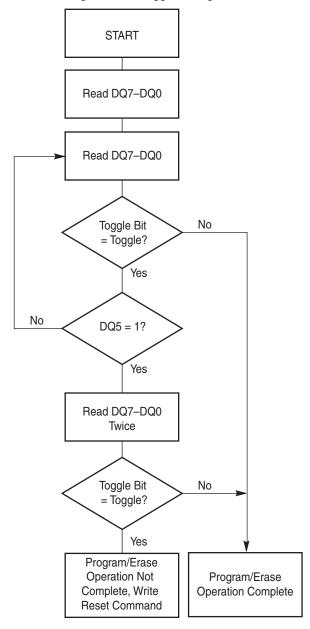
Figure 10.6 Toggle Bit Algorithm
