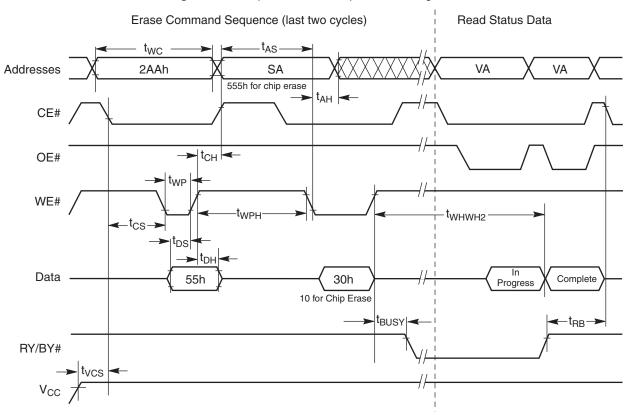
Figure 15.7 Chip/Sector Erase Operation Timings
