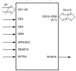
Figure 5.5 S29GL032N Logic Symbol (Models 03, 04)
