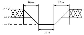
Figure 11.2 Maximum Positive Overshoot Waveform
