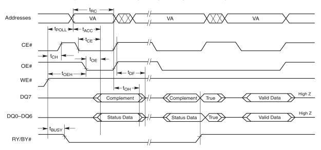
Figure 15.8 Data# Polling Timings (During Embedded Algorithms)
