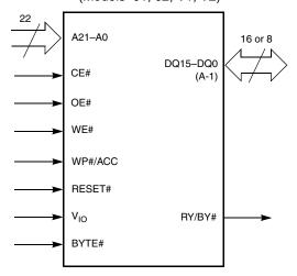
**Figure 5.3** S29GL064N Logic Symbol (Models 06, 07, V6, V7)
