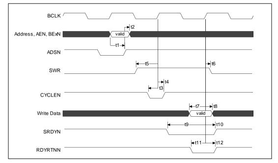
Figure 22. Synchronous Write Cycle – VLBUSN = 0
