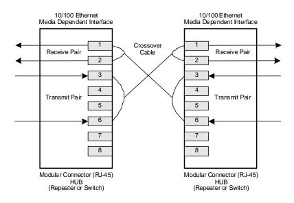
Figure 7. Typical Crossover Cable Connection
