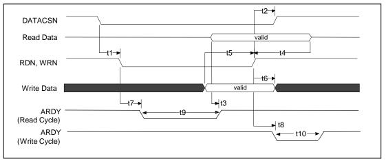
Figure 18. Asynchronous Cycle – Using DATACSN
