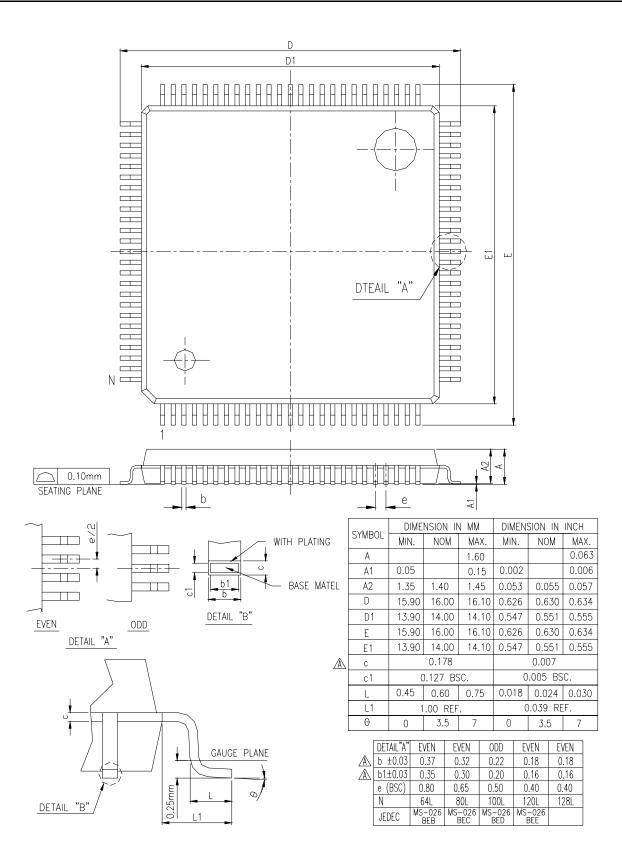
Figure 28. Optional 128-Pin LQFP Package
