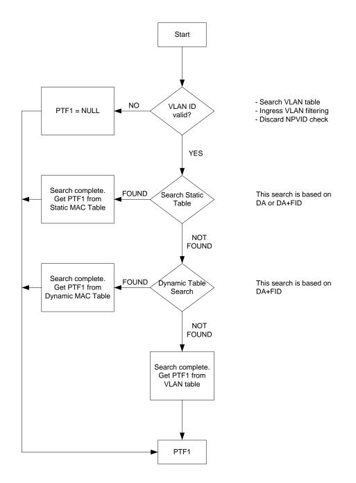
Figure 9. Destination Address Lookup Flow Chart in Stage One
