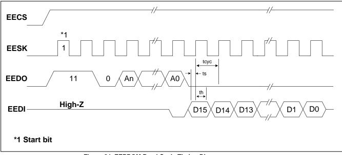
Figure 24. EEPROM Read Cycle Timing Diagram
