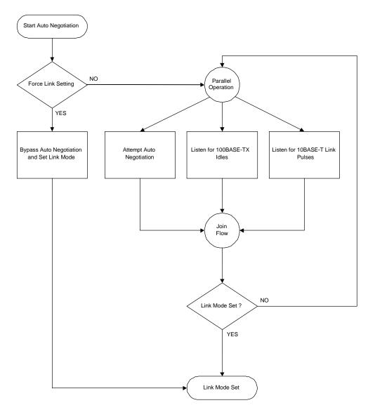
Figure 8. Auto Negotiation and Parallel Operation
