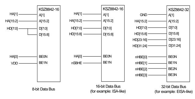
Figure 12. KSZ8842M 8-Bit, 16-Bit, and 32-Bit Data Bus Connections
