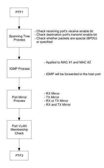
Figure 10. Destination Address Resolution Flow Chart in Stage Two
