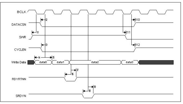
Figure 20. Synchronous Burst Write Cycles – VLBUSN = 1
