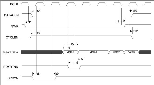
Figure 21. Synchronous Burst Read Cycles – VLBUSN = 1
