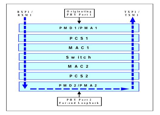
Figure 14. Port 2 Far-End Loopback Path
