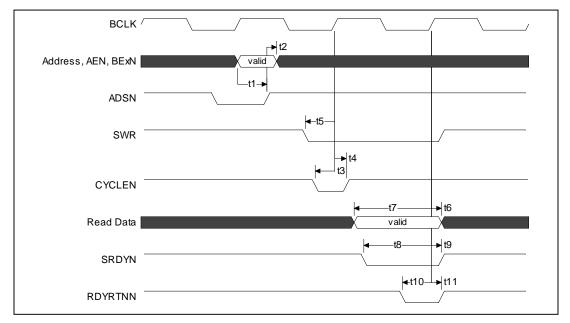
Figure 23. Synchronous Read Cycle – VLBUSN = 0
