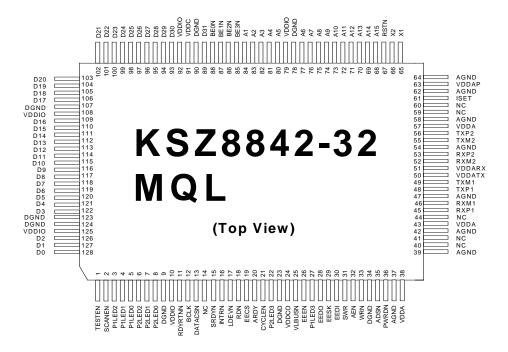
Figure 4. Standard – KSZ8842-32 MQL 128-Pin PQFP (Top View)
