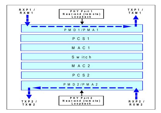
Figure 15. Port 1 and port 2 Near-End (Remote) Loopback Path
