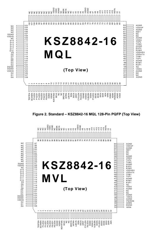
Figure 3. Option - KSZ8842-16 MVL 128-Pin LQFP (Top View)
