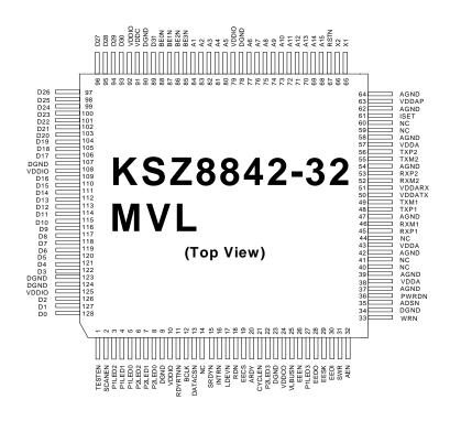
Figure 5. Option – KSZ8842-32 MVL 128-Pin LQFP (Top View)
