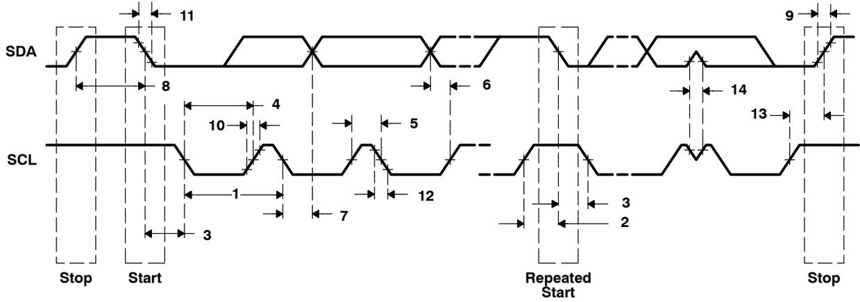
Figure 51. I<sup>2</sup>C Receive Timings
