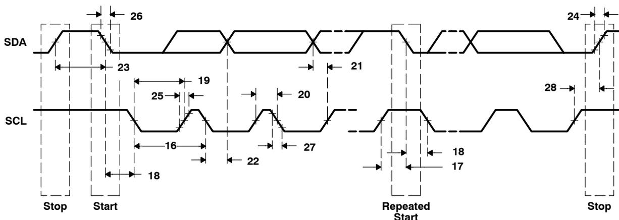
Figure 52. I<sup>2</sup>C Transmit Timings
