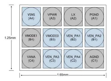
Note: VEN\_PA4 will be treated as VEN\_DC in the configuration with three (3) PAs and a seperate DC-DC Enable.
