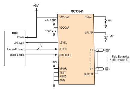
Figure 6. Simplified Application Diagram
