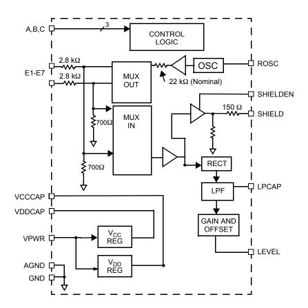
Figure 1. Simplified Functional Block Diagram
