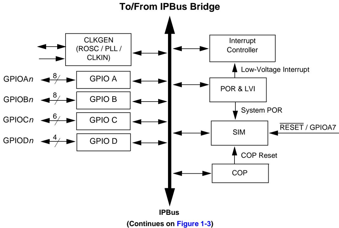
**Figure 1-2 Peripheral Subsystem**
