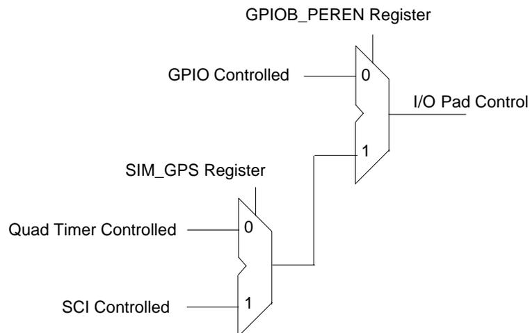
**Figure 6-9 Overall Control of Pads Using SIM\_GPS Control**
