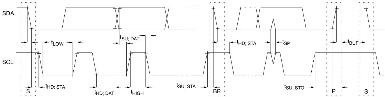
Figure 10-14 Timing Definition for Fast and Standard Mode Devices on the I<sup>2</sup>C Bus
