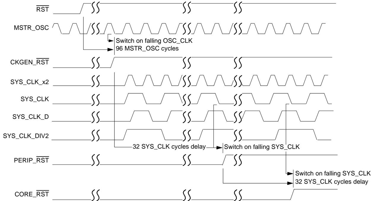
Figure 6-16 Timing Relationships of Reset Signal to Clocks
