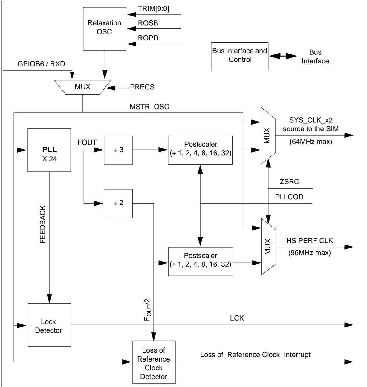
Figure 3-2 OCSS Block Diagram with Relaxation Oscillator
