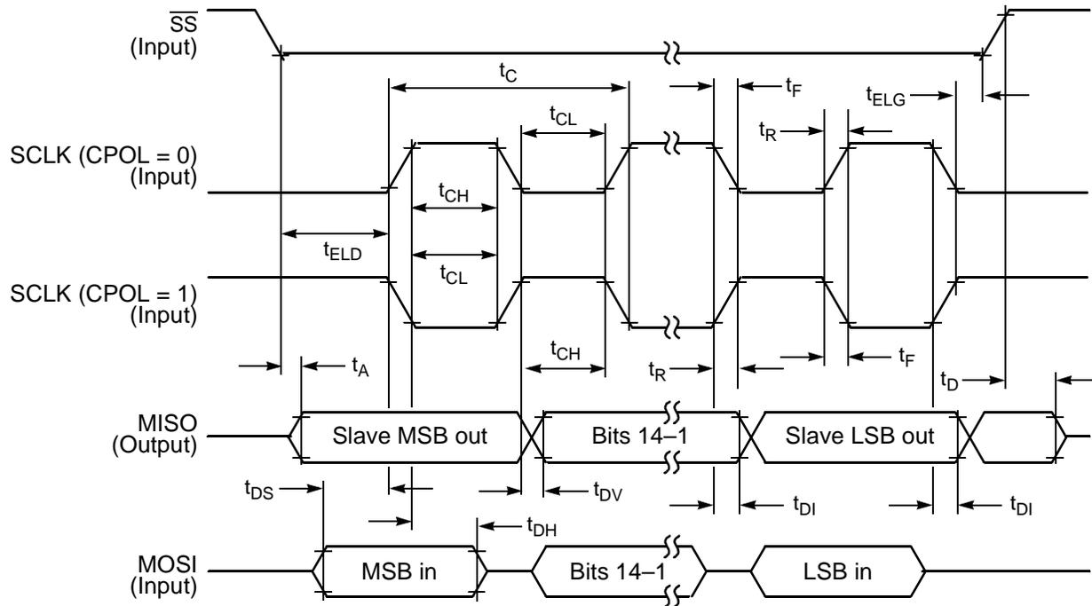
**Figure 10-9 SPI Slave Timing (CPHA = 0)**
