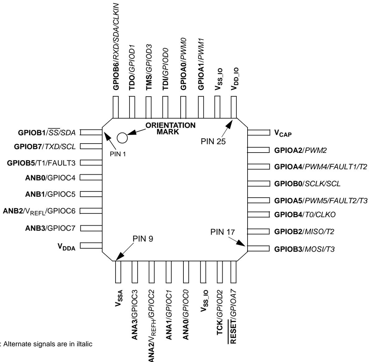
Figure 11-1 Top View, 56F8014 32-Pin LQFP Package
