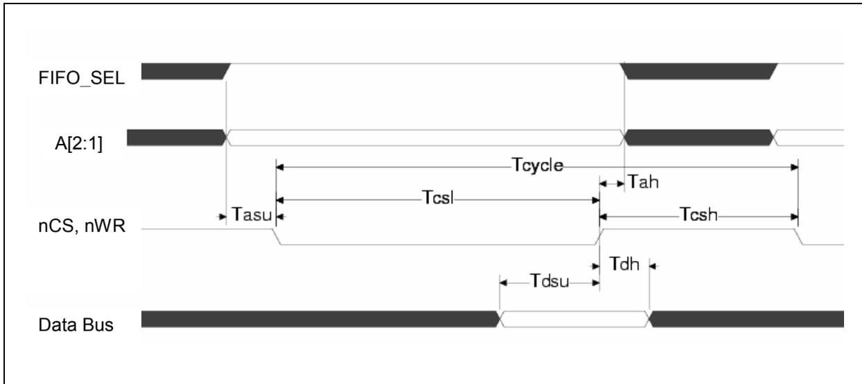
**Figure 6.7 TX Data FIFO Direct PIO Write Timing**
