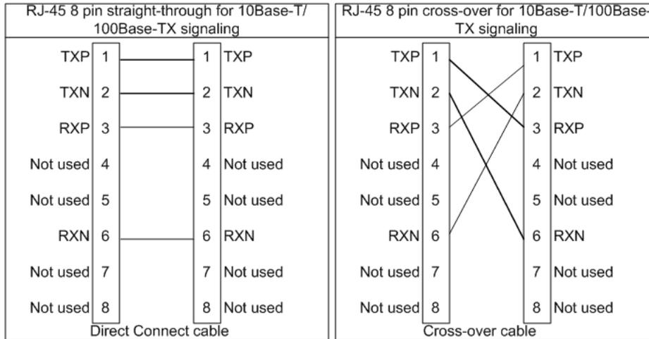
**Figure 4.3 Direct cable connection vs. Cross-over cable connection.**
