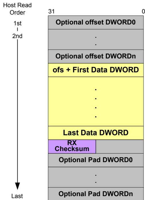
Figure 3.21 RX Packet Format with RX Checksum
