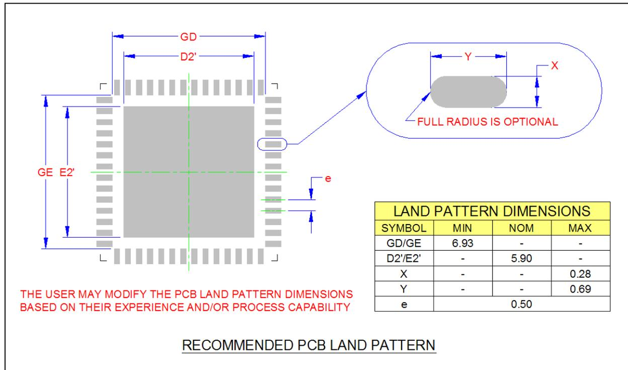
Figure 8.2 56 Pin QFN Recommended PCB Land Pattern
