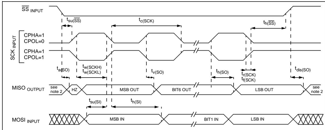
Figure 92. SPI Master Timing Diagram <sup>1)</sup>
