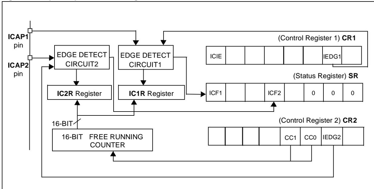
Figure 41. Input Capture Timing Diagram
