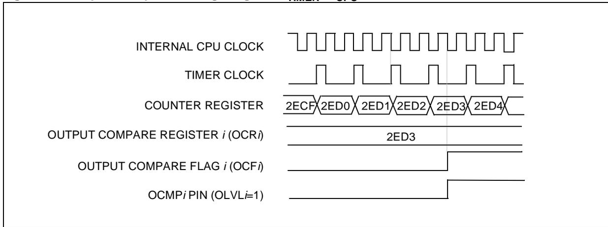
Figure 44. Output Compare Timing Diagram,  $f_{\text{TIMER}} = f_{\text{CPU}}/4$
