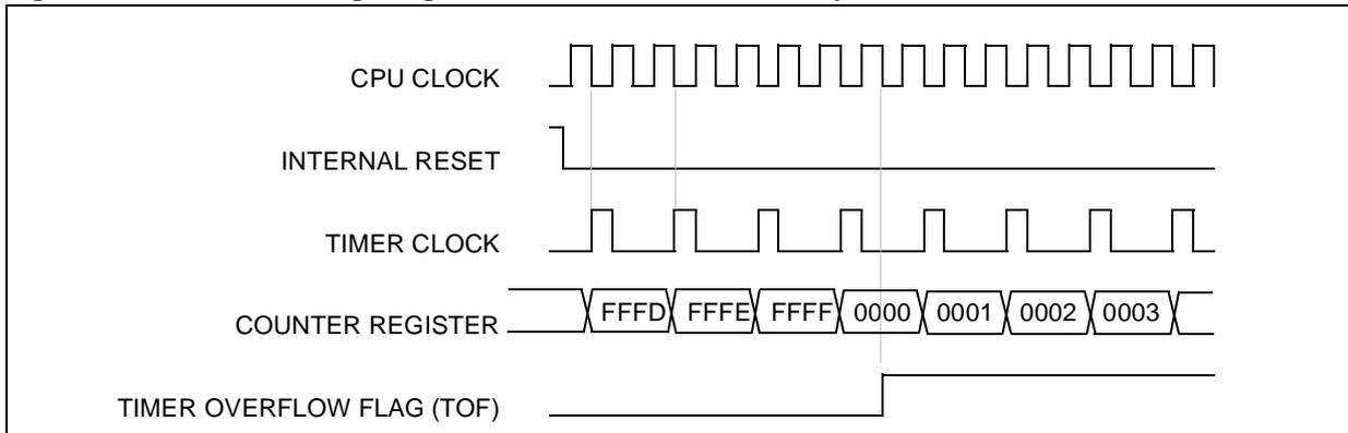
Figure 38. Counter Timing Diagram, internal clock divided by 4
