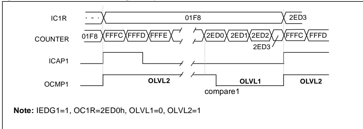
Figure 46. Pulse Width Modulation Mode Timing Example with 2 Output Compare Functions
