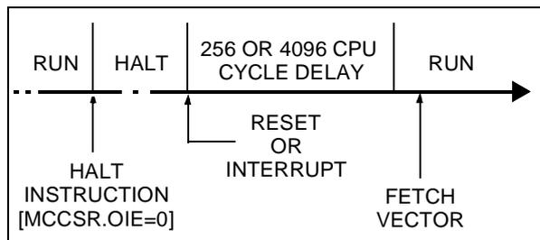
**Figure 29. HALT Mode Flow-chart**
