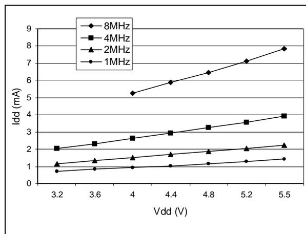
Figure 64. Typical I<sub>DD</sub> in SLOW vs. f<sub>CPU</sub>
