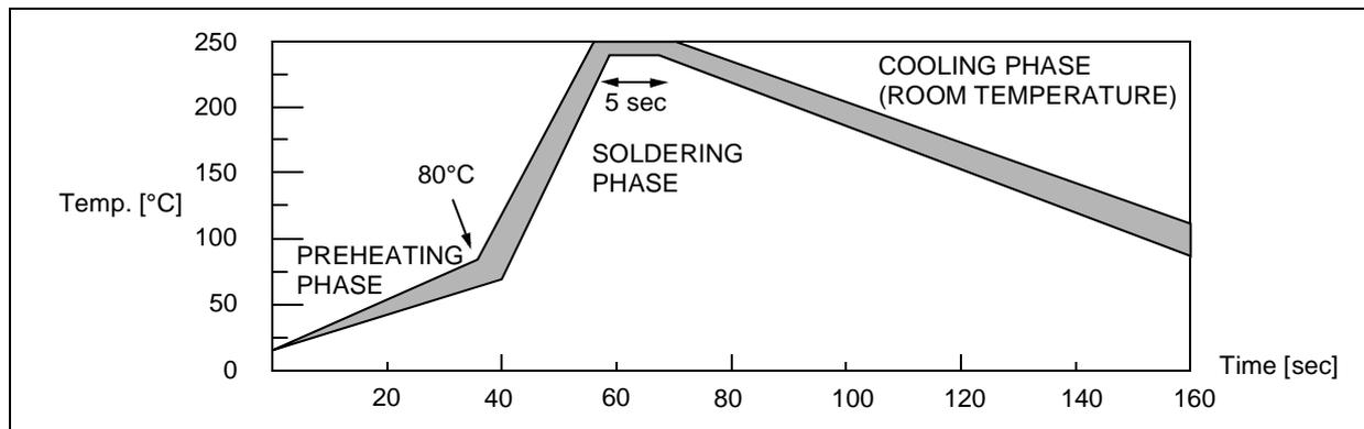
**Figure 103. Recommended Reflow Soldering Oven Profile (MID JEDEC)**
