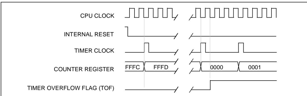
Figure 39. Counter Timing Diagram, internal clock divided by 8
