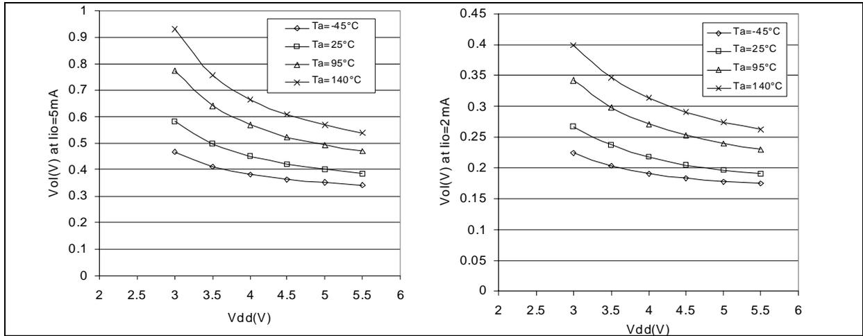
Figure 86. Typical  $V_{OL}$  vs.  $V_{DD}$  (high-sink)
