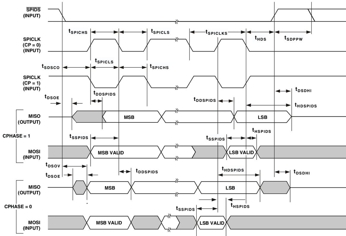
Figure 26. SPI Protocol—Slave
