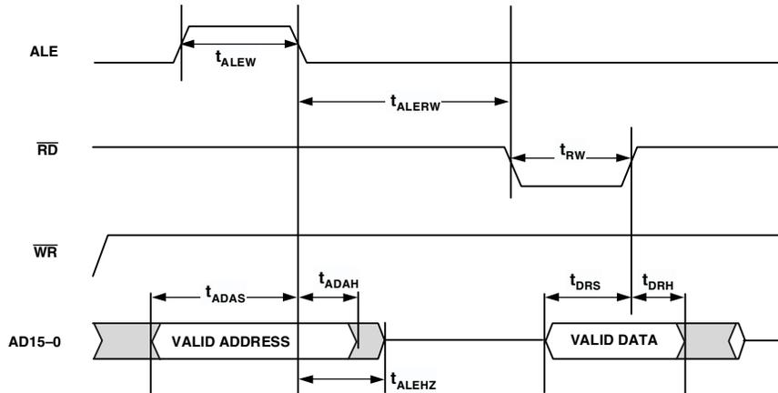
Figure 18. 16-Bit Memory Read Cycle
