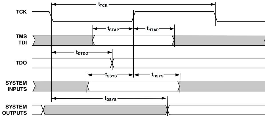
Figure 27. JTAG Test Access Port and Emulation
